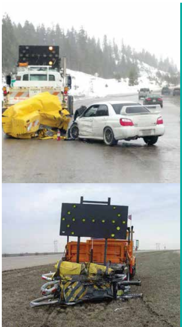
Figure 37. A TMA following impact by an automobile (Image: Traffix Devices Inc.)
