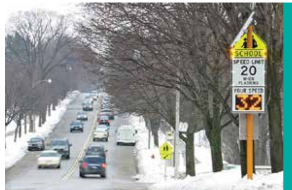
Figure 9. A speed indicator board provides instant feedback to the driver (Image: TAPCO)
